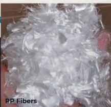
preventing and suppressing crack formation, significantly boosting anti-crack, anti-seepage,, antiimpact. and anti-seismic capabilities. The versatility of these fibers extends to various applications, including underground waterproofing, roofing, walls, industrial and civil construction projects, pools, basements, roads, and bridges.
